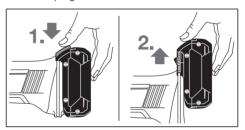
To remove the battery **5**, press the unlocking button **6** and pull out the battery toward the front. **Do not exert any force.**
