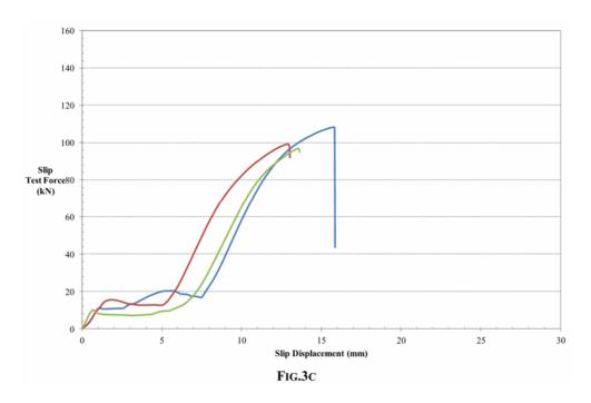
Shear Load vs Displacement Curve ORB2020B Longitudinal Vertically aligned downwards bolt at extremity of slot 16mm plate thickness, M20 x 60mm bolt
