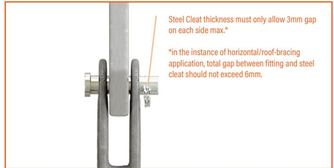
1. ReidBar™ is tightly fastened into the RBRACE-END fitting.
