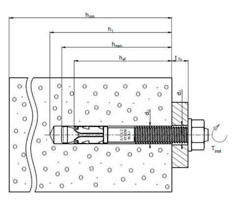
h<sub>min</sub> : Minimum thickness of concrete member
