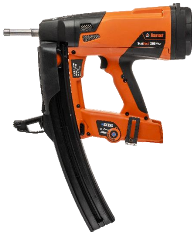
TrakFast™ 800 Plus (100 Joules) for pins up to 32 mm length
