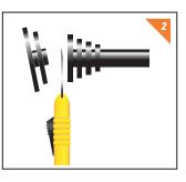
2. Cut Piston Pug to suit desired hole size. For deeper holes, a 10mm clear vinyl extension tube can be fitted to the nozzle, cut to the required length, with the piston plug secured at the opposite end.
