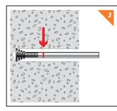
3. Attach Piston Plug to the end of the tubing and then mark 1/4 embedment depth on the flexible tubing.
