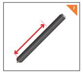
1. Measure embedment depth and then cut the 10mm vinyl tube to that length.
